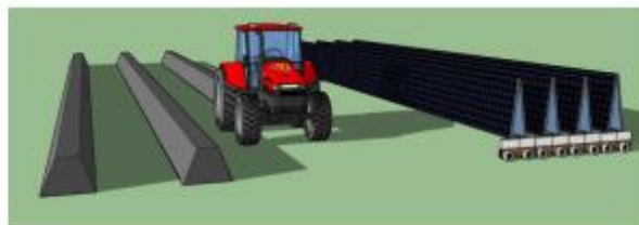
Fig. 3: The wheel-rail based design makes it easy to fold the PV structure together when farming practices are needed (in this figure, as example, beds are created).
